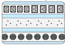
IEC and UK / Schuko / FR outlets can be configured in a single PDU in order to increase the compatibility to different power cords of the rack mount equipment.
