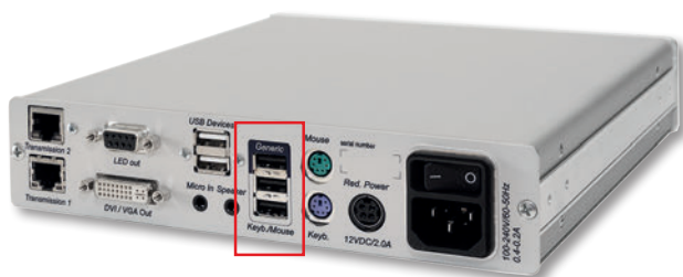
Back panel of DVI-U-CON-2 with Generic USB interface and additional interface for transparent USB transmission
