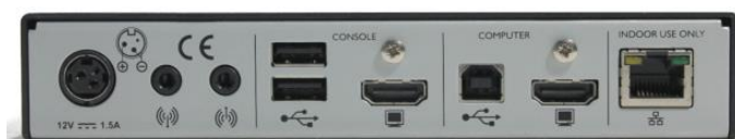
UltraLink 2 HDMI – rear panel
