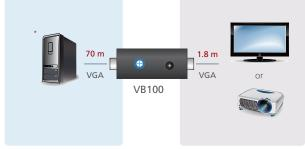
\* If the source device cannot power the VB100 please use the power adapter included with this package.
